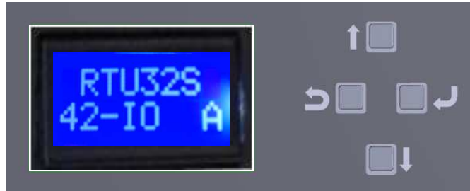
Figure 18: Display and Keys on the RTU32S Front Panel
