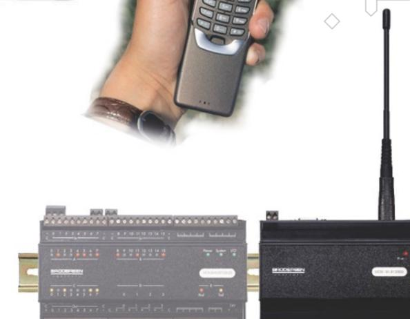
GSM Modem fitted on DIN rail next to Brodersen compact outstation RTU8
