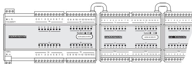
In the event that the current consumption of the expansion modules exceeds the capability of the power supply, an additional power supply must be inserted.
